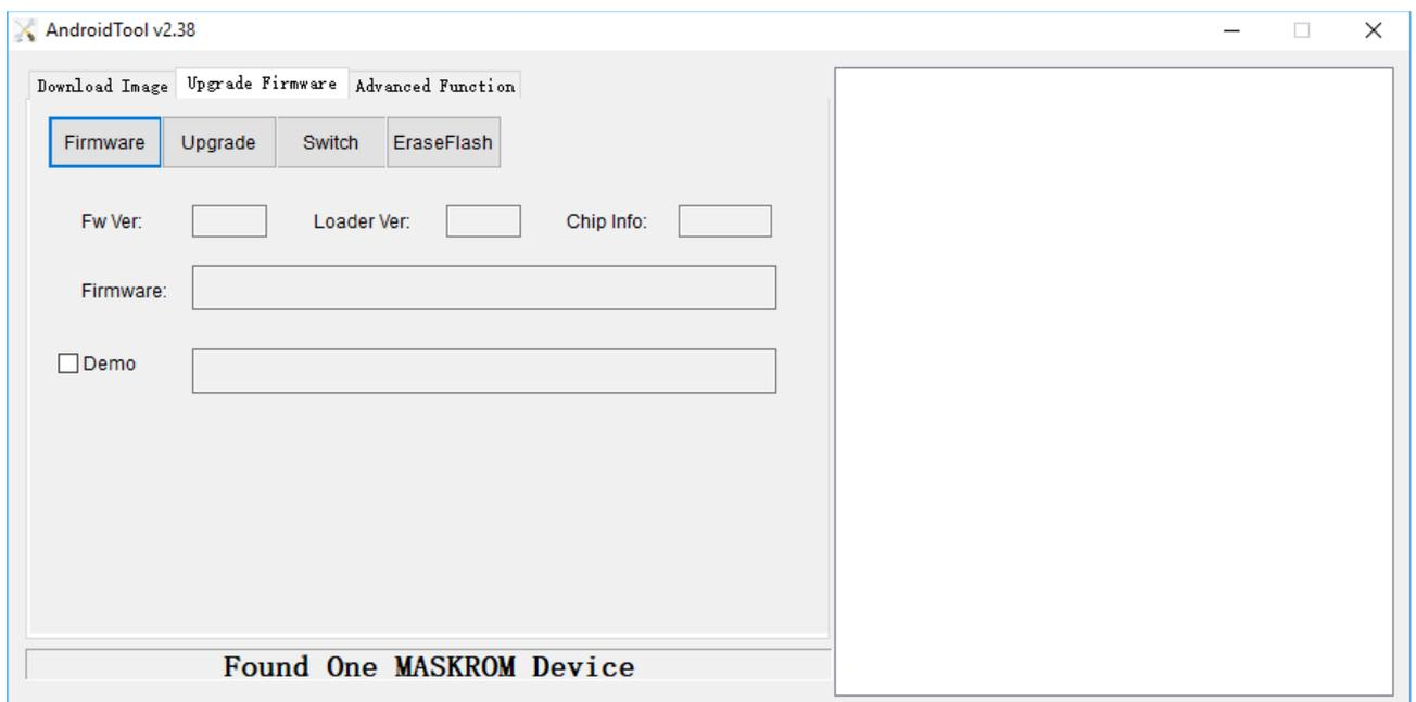
**STEP 04** Remove the jumper from the ROCK64 board after you see the “Found One MASKROM Device” message in AndroidTool.exe
