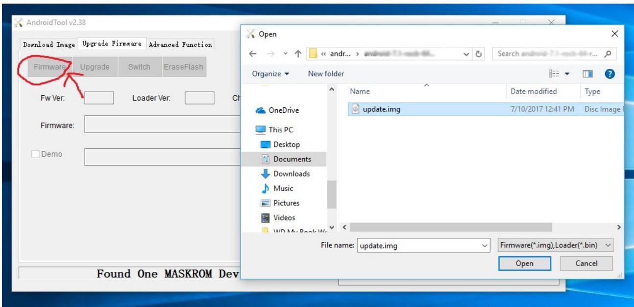
Click the Upgrade section to start flashing the Android firmware into eMMC
