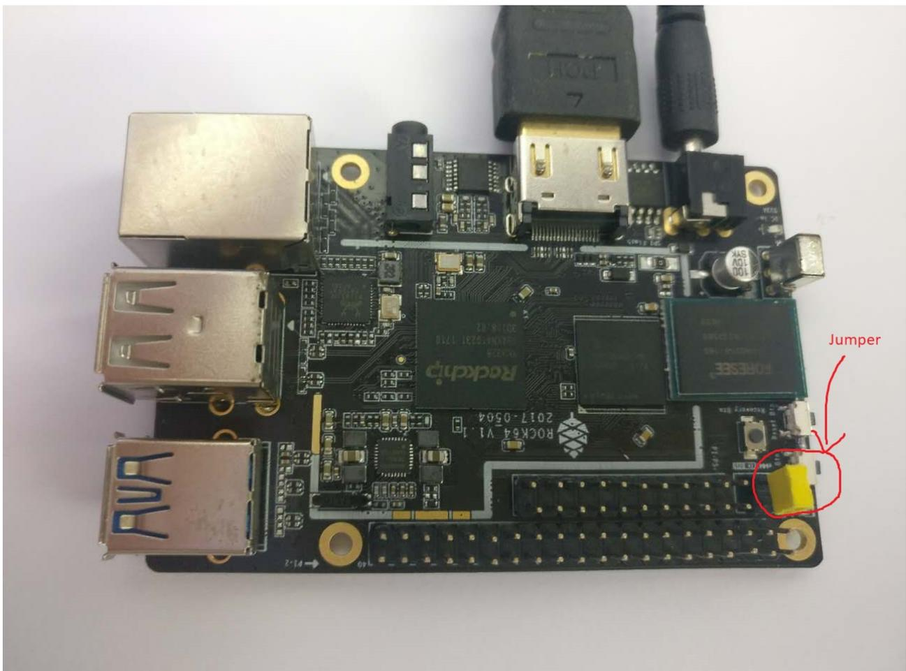
3. Connect USB A-to-A cable to upper USB 2.0 port of ROCK64 board and your computer's USB port.
