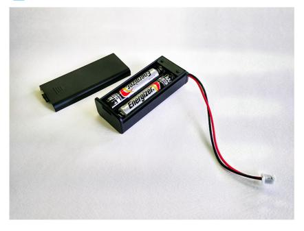
**STEP 02** Tighten the battery compartment cover of RTC Backup Battery Holder. Connect the RTC Backup Battery Holder to RTC port on PINE A64. Turn ON the power switch on the holder to start.
