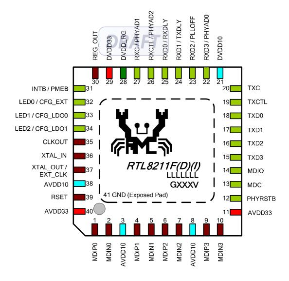
Figure 4. Pin Assignments (40-Pin QFN)
