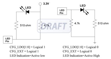
Figure 5. LED and PHY Address Configuration
