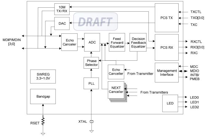
Figure 3. Block Diagram
