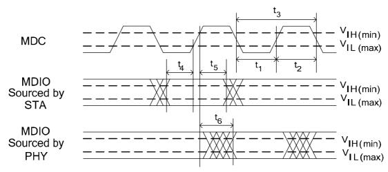
Figure 26. MDC/MDIO Management Timing Parameters
