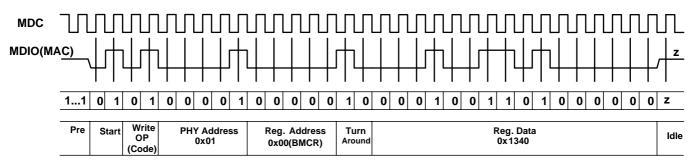
Figure 7. MDC/MDIO Write Timing
