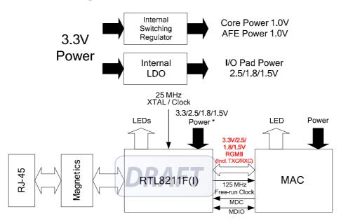
\*Note: 3.3/2.5/1.8/1.5V power here means I/O pad power sourced from external power, not from the internal LDO.
