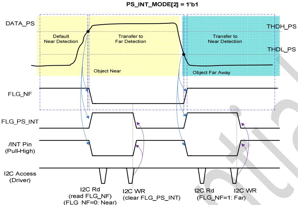
PS persistence numbers PRST\_PS[1:0] is used to avoid the false alarm of PS interrupt event due to environment noise. If PS persistence is set larger than 1, then the PS interrupt will not be issued until continuous persistence numbers of ADC conversion results meet the interrupt condition describe above.
