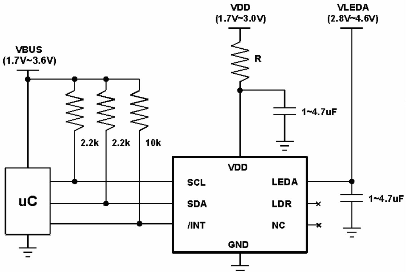
STK3335 Typical Application Circuit with Independent VDD and VLED Supply Voltage
