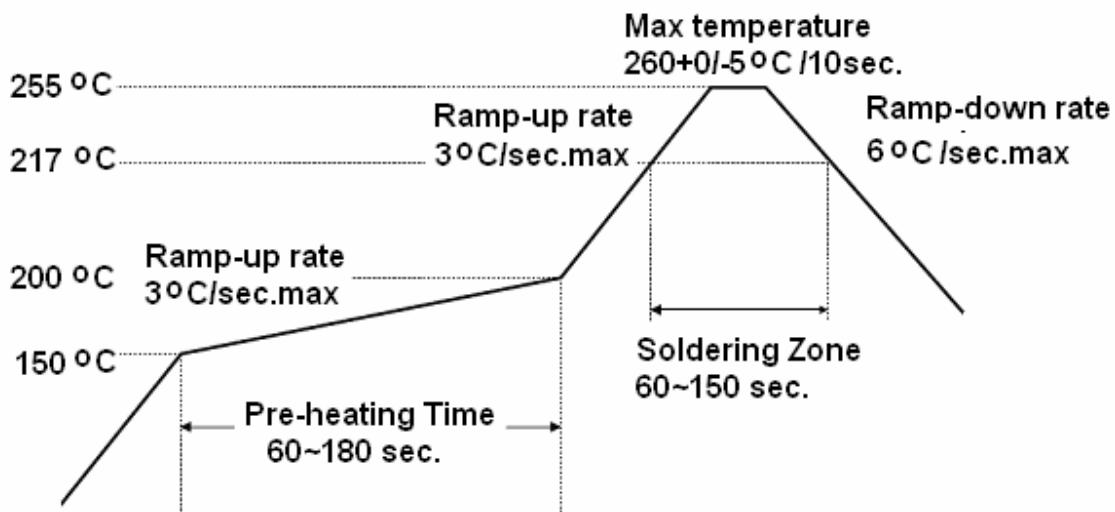
2. Reflow soldering should not be done more than three times.
