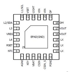
Fig 2 IP5209 Pin Diagram
