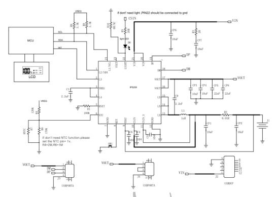
Fig 8 Typical application schematic with I2C
