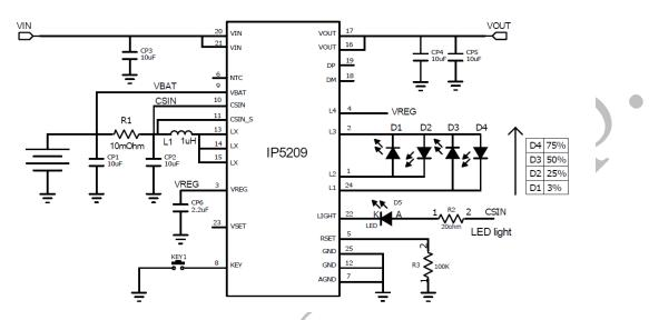
Fig 1 Simplified application schematic (4 LEDs as the SOC indicator)
