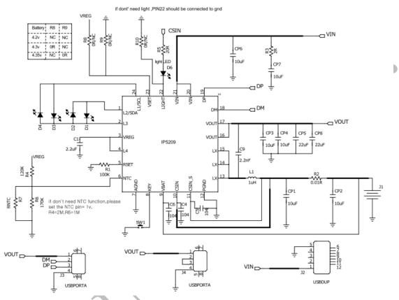
Fig 7 4 LEDs SOC indicator typical application schematic
