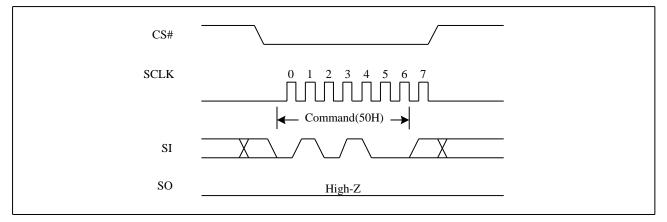
Figure5a. Write Enable for Volatile Status Register Sequence Diagram (QPI)
