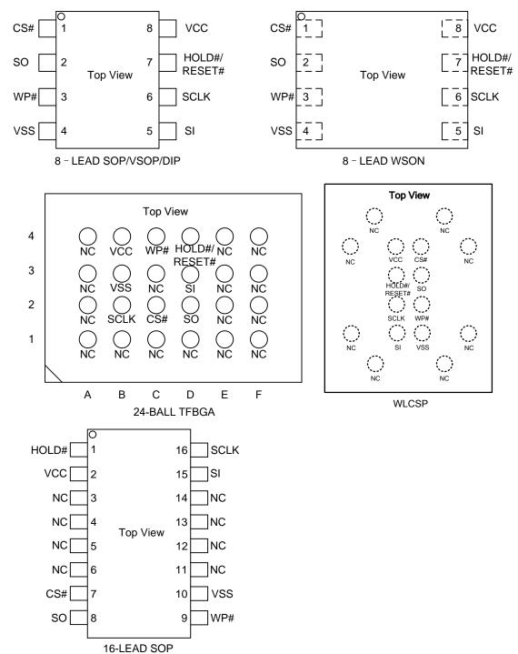
Note: Only for special order, Pin 3 is RESET# pin. Please contact GigaDevice for detail.
