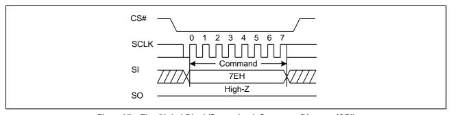
Figure37a. The Global Block/Sector Lock Sequence Diagram (QPI)
