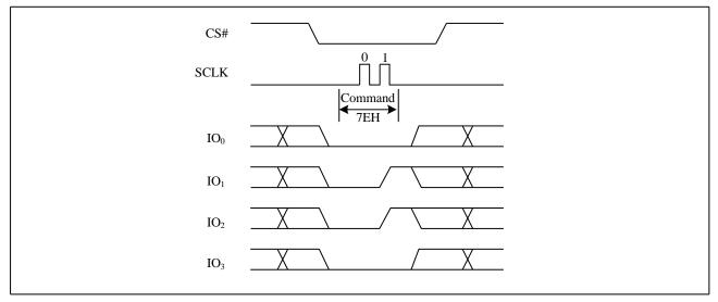
Figure 38. The Global Block/Sector Unlock Sequence Diagram
