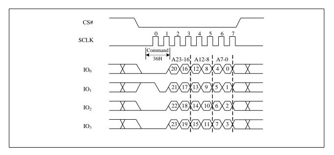
Figure 35. Individual Block/Sector Unlock command Sequence Diagram
