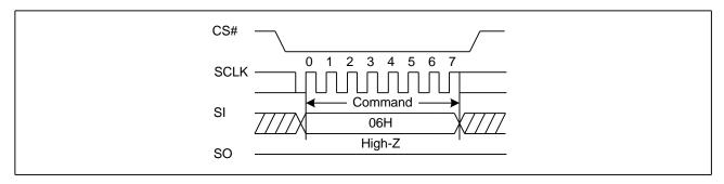
Figure3a. Write Enable Sequence Diagram (QPI)
