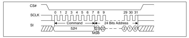
Figure19a. 32KB Block Erase Sequence Diagram (QPI)
