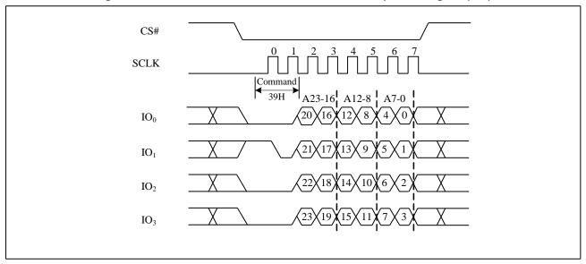
Figure 36. Read Individual Block/Sector lock command Sequence Diagram
