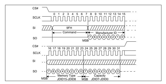
Figure 28. Read Identification ID Sequence Diagram
