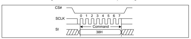
Figure 41. Enable QPI mode command Sequence Diagram
