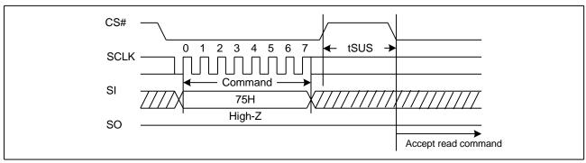
Figure 29. Program/Erase Suspend Sequence Diagram
