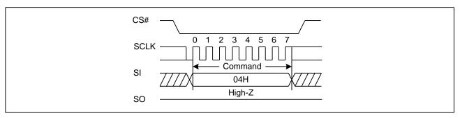
Figure 4a. Write Disable Sequence Diagram (QPI)
