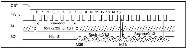
Figure6a. Read Status Register Sequence Diagram (QPI)
