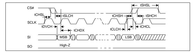
Figure 50. Output Timing
