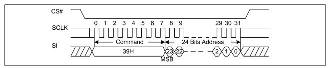
Figure35a. Individual Block/Sector Unlock command Sequence Diagram (QPI)
