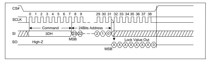
Figure36a. Read Individual Block/Sector lock command Sequence Diagram (QPI)
