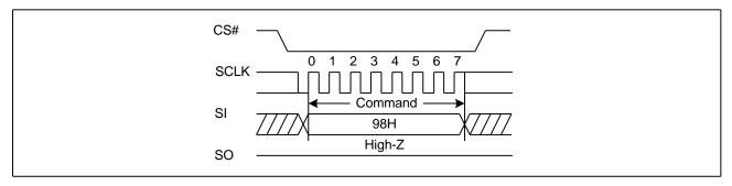
Figure38a. The Global Block/Sector Unlock Sequence Diagram (QPI)
