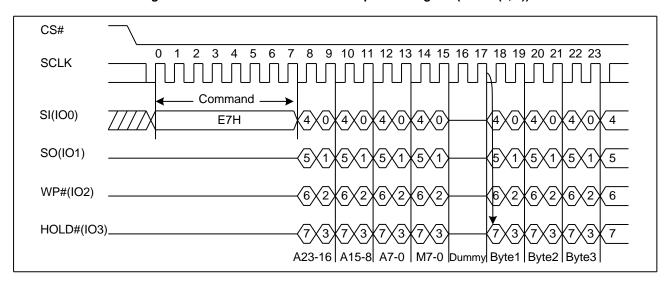
Figure 14. Quad I/O Word Fast Read Sequence Diagram (M5-4≠ (1, 0))
