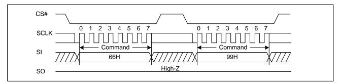
Figure 44. Enable Reset and Reset command Sequence Diagram (QPI)
