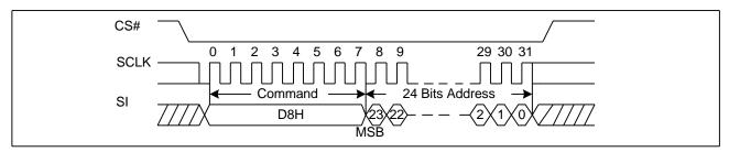
Figure 20a. 64KB Block Erase Sequence Diagram (QPI)
