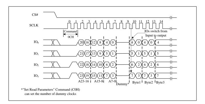
Figure 40. Burst Read with Wrap command Sequence Diagram
