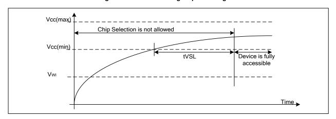
Table 8.1. Power-Up Timing and Write Inhibit Threshold
