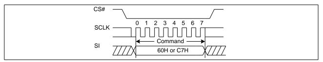
Figure21a. Chip Erase Sequence Diagram (QPI)
