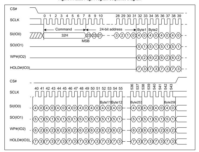
Figure 17. Quad Page Program Sequence Diagram
