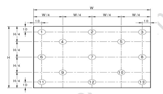
The White luminance uniformity on LCD surface is then expressed as :  $\Delta$ Y5 = Minimum Luminance of five points / Maximum Luminance of five points (see FIGURE 2),  $\Delta$ Y13 = Minimum Luminance of 13 points /Maximum Luminance of 13 points (see FIGURE 3).
