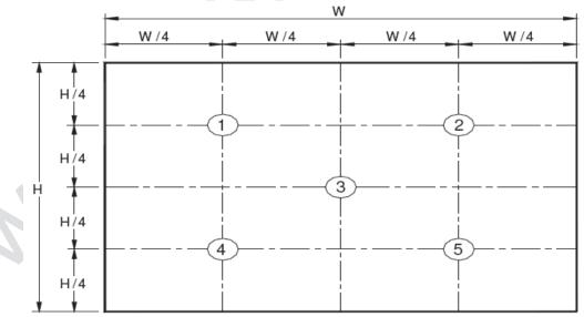
Center Luminance of white is defined as luminance values of center 5 points across the LCD surface. Luminance shall be measured with all pixels in the view field set first to white. This measurement shall be taken at the locations shown in FIGURE 2 for a total of the measurements per display.
