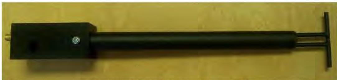
Figure 1 – MVG COMOSAR Validation Dipole
