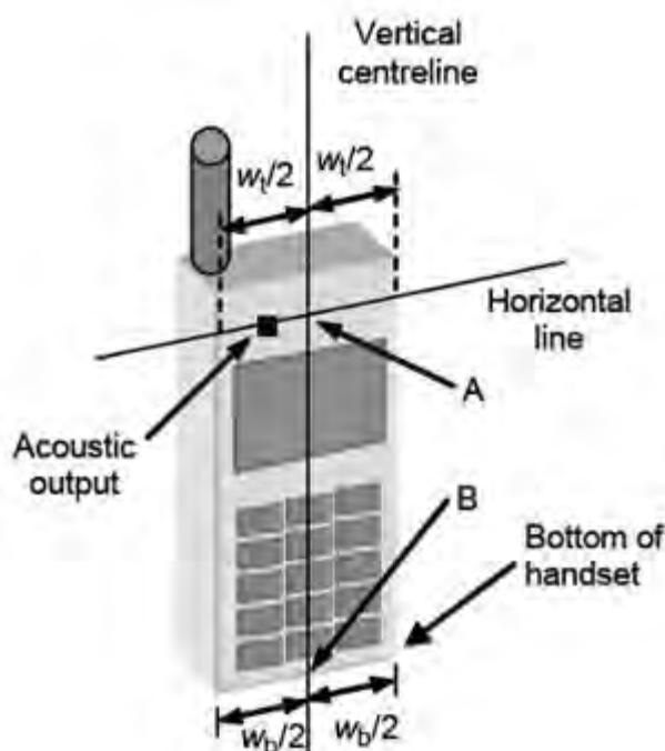
Fig 6.2.1 Handset vertical and horizontal reference lines—fixed case
