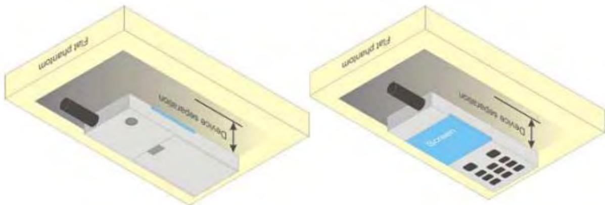
Figure 6.4.1 – Test positions for body-worn devices
