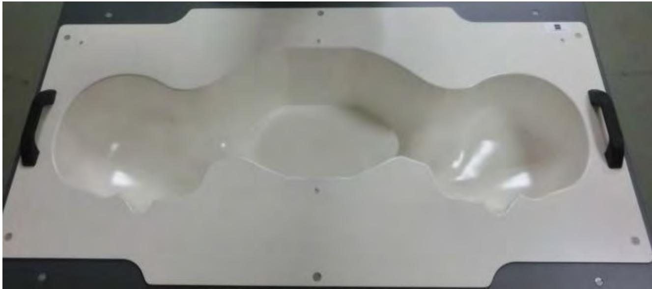
The SAM phantom is used to measure the SAR relative to people exposed to electro-magnetic field radiated by mobile phones.
