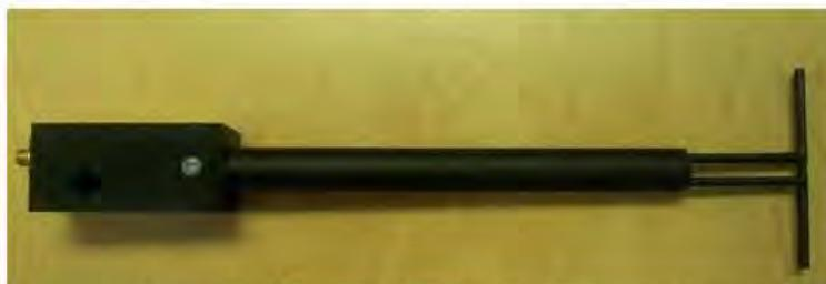
Figure 1 – MVG COMOSAR Validation Dipole
