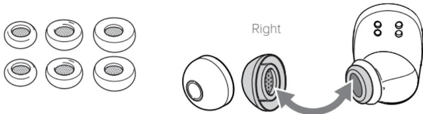
When attaching new eartips, ensure the oval mounting tip on the earbud is aligned with the oval attachment on the eartips. Press the eartips firmly onto the ear.
