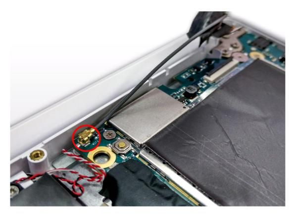
**STEP 04** Undo the hinges on both sides and the screen connector located on the main board. The hinges are held in place with Philips screws.
