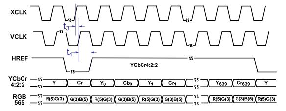
Figure 5. Horizontal Timing YUV4:2:2
