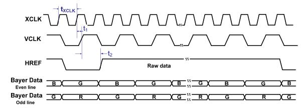
Figure 4. Horizontal Timing Raw Bayer Data
