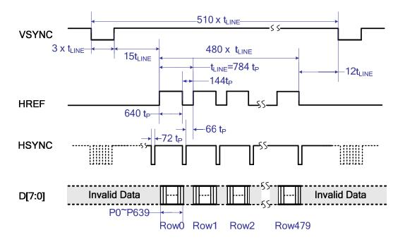
Figure 6. VGA Frame Timing
