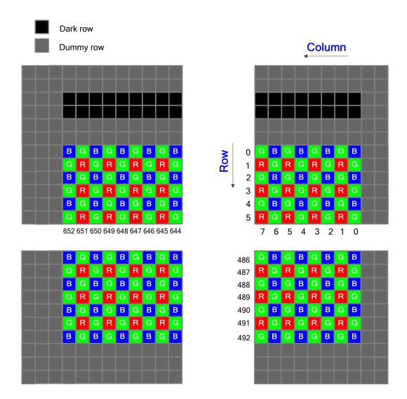
Figure 2. Sensor Array Region
