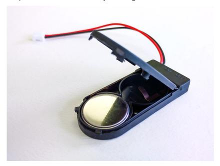
**STEP 04** Tighten the battery compartment cover of RTC Backup Battery Holder. Connect the RTC Backup Battery Holder to RTC port on PINE A64
