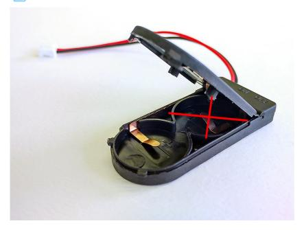
**STEP 02** Get a CR2032 3V Battery from a retail shop (to be inserted into RTC Backup Battery Holder)
