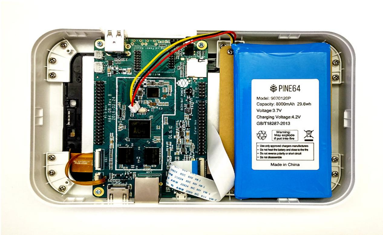
**STEP 06** Insert the balance wire of the lithium polymer battery into the balance connector on PINE A64.
