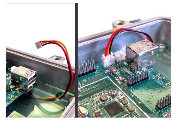
**STEP 09** Now, assembly the case and the base of the aluminum waterproof enclosure.
