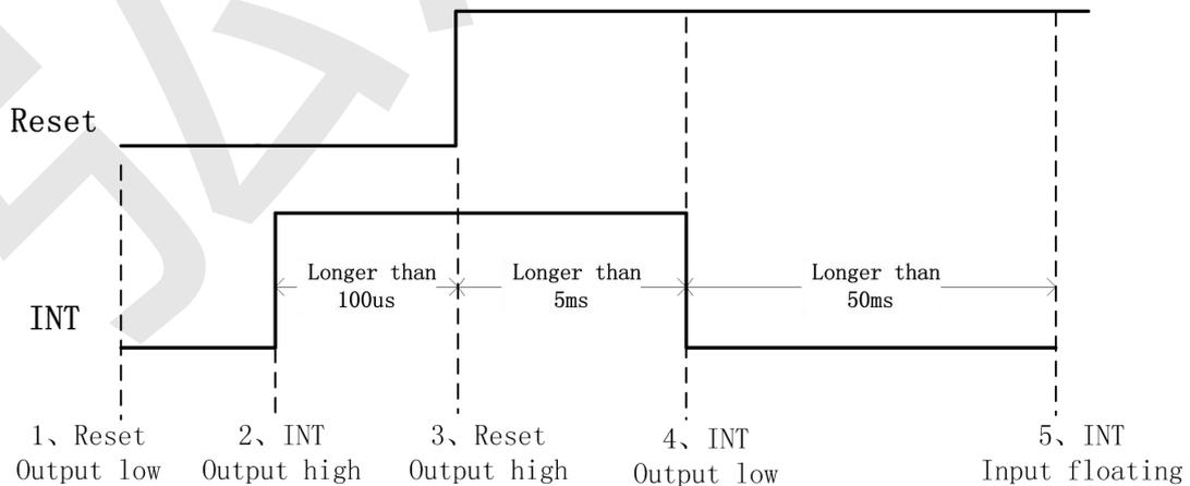
**Timing for setting slave address to 0xBA/0xBB:**
